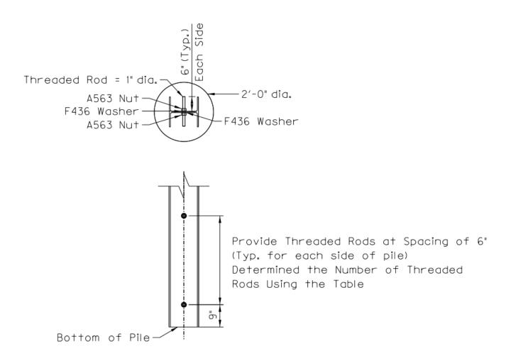
Figure 1: Threaded rod detail
